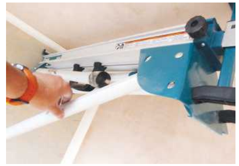
▲ The pins are sprung to lock open or closed for easy deployment
